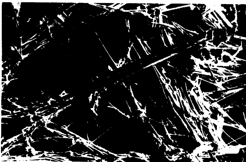
Fig. 3. SEM micrograph showing needle-like crystals of K up to 10 \mu m long.
