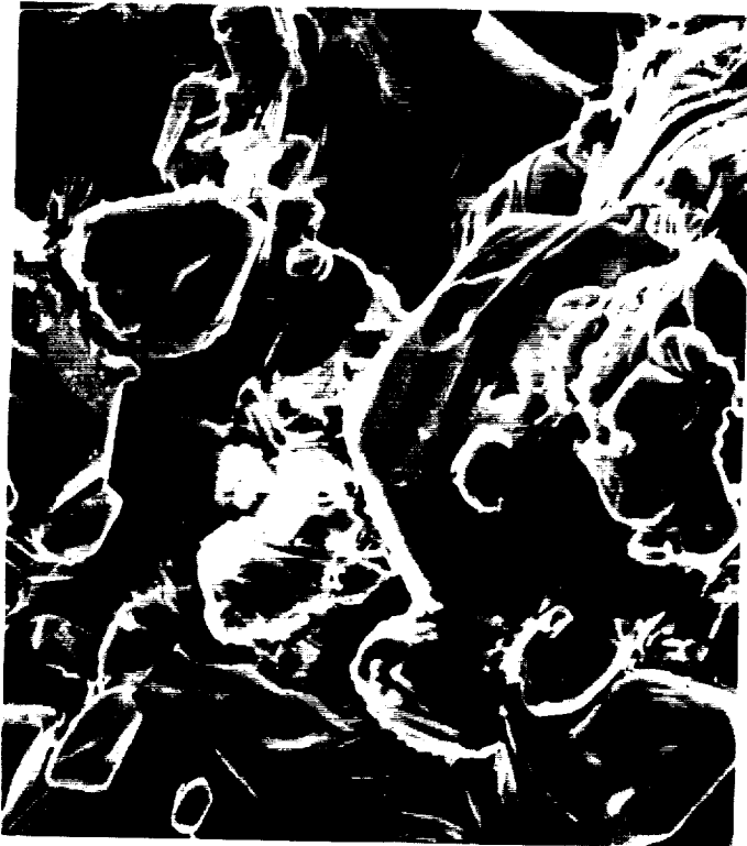
Figure 8. When superconductors were stacked for firing, the lower one showed glitter so we took a look at a) 500X SEM, and b) 1500X SEM. Note the planes within the crystals.
