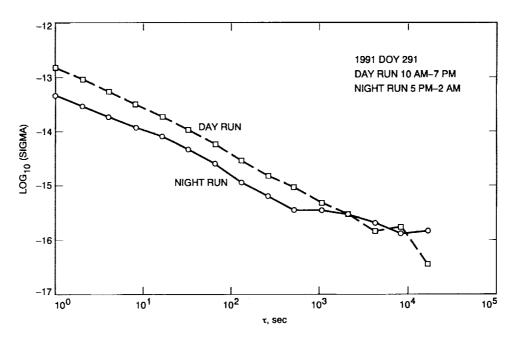
Fig. 8. Alian deviation characteristics of the 12-GHz fiber-optic system for day and night runs on 1991 DOY 291. The signal source was driven by 5 MHz from a portable Cesium reference standard. Test frequency was 12.248 GHz.
