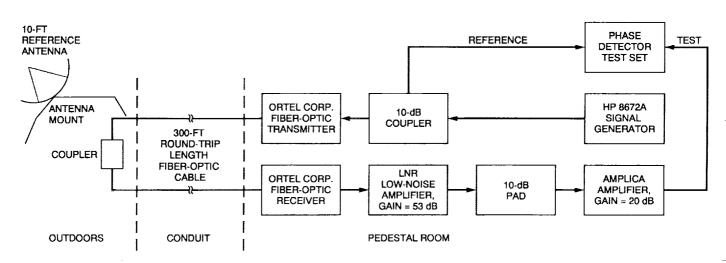
Fig. 4. Block diagram of the measurement setup to test the 12-GHz fiber-optic system that was installed at DSS 13.
