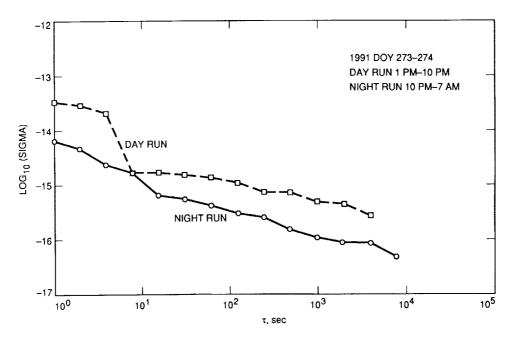
Fig. 5. Allan deviation characteristics of the 12-GHz fiber-optic system for day and night runs on 1991 DOY 273–274. The signal source was free-running. Test frequency was 12.198 GHz.
