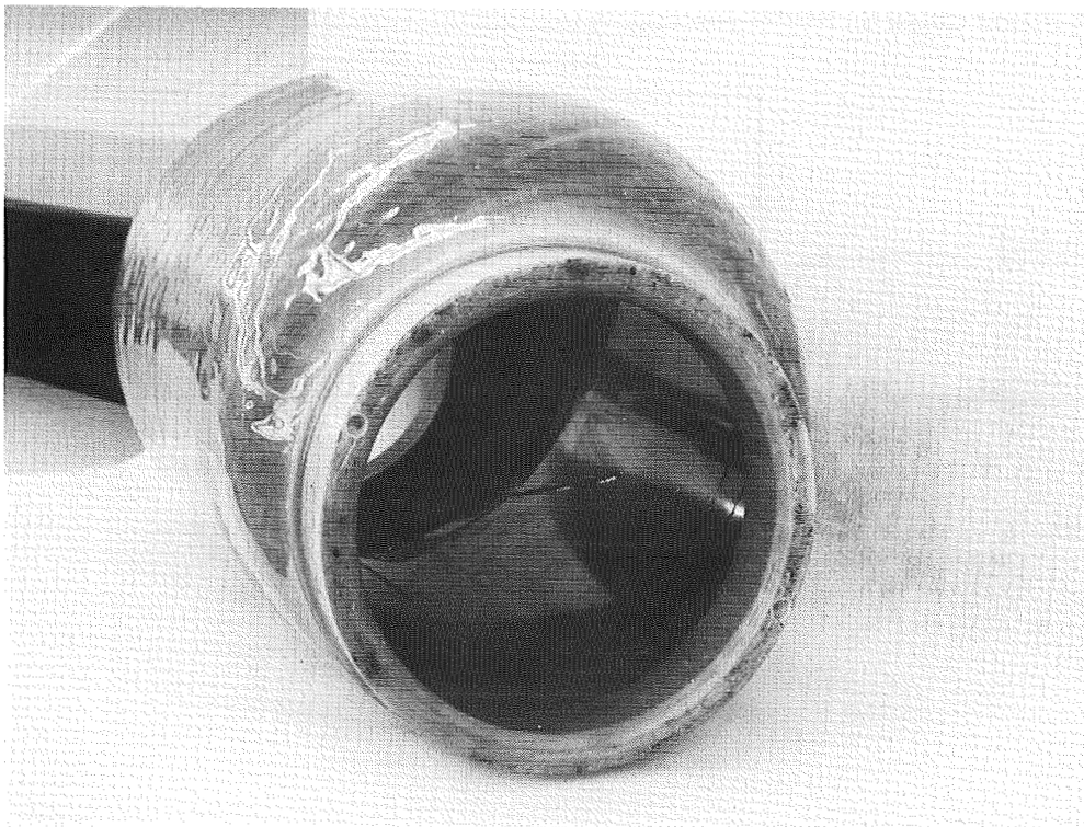
Figure 9. Bore evacuator chamber.
