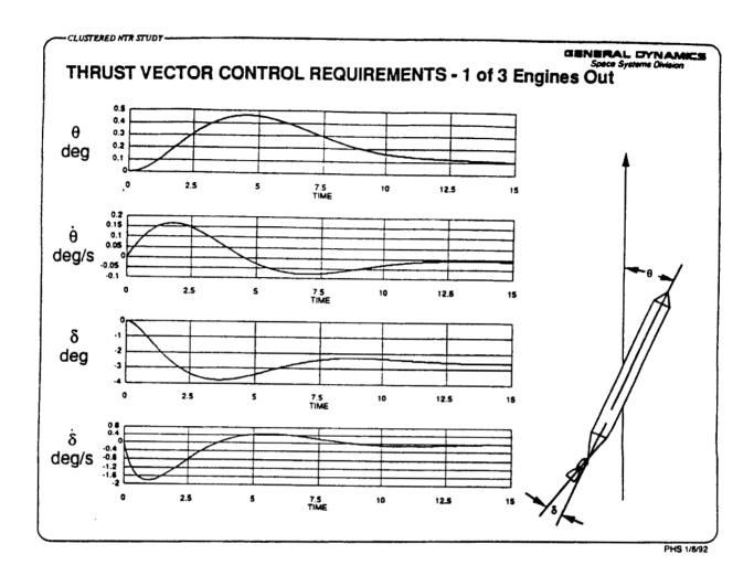
A dynamic guidance and control simulation was developed to examine the vehicle control response and engine gimballing requirements for the case where one engine of 3 fails. The vehicle mass distribution was examined and it was concluded that the worst case could be approximated with the Mars transfer injection maneuver tanks jettisoned and the aft core tank full of propellant. Instantaneous shutdown of the faulted engine also was assumed for the worst case.
