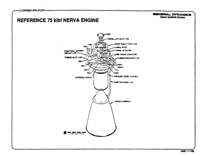
The reference engine is a NERVA "full flow" concept developed by Altseimer of Aerojet Nuclear Systems Company, circa 1971. It is an engine typical of that era. For the two engine cases, the reference 75 klbf engine was used, the three engine cases utilized a scaled down version of this engine sized at 50 klbf.
