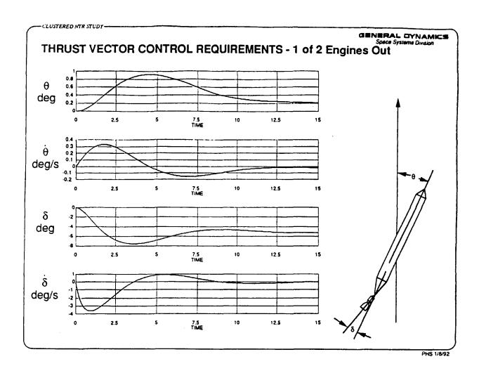
A dynamic guidance and control simulation was developed to examine the vehicle control response and engine gimballing requirements for the case where one engine of 2 fails. The vehicle mass distribution was examined and it was concluded that the worst case could be approximated with the Mars transfer injection maneuver tanks jettisoned and the aft core tank full of propellant. Instantaneous shutdown of the faulted engine also was assumed for the worst case.
