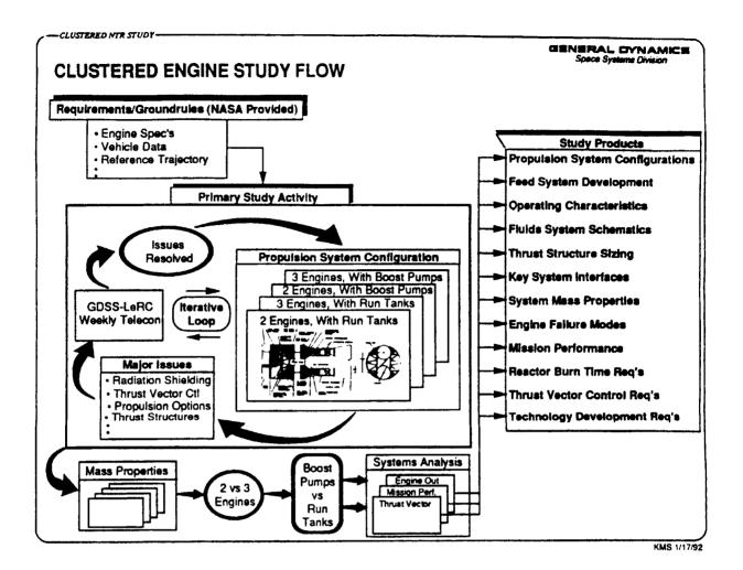
The study was initiated with a series of NASA LeRC provided groundrules and requirements. These were provided in appendix form and served as the point of departure for the NTP vehicle, mission, engine and propulsion system.
