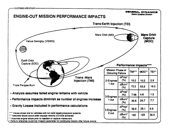
A Mars Transfer System(MTS) with multiple nuclear thermal rocket engines departs from earth parking orbit on 150-day trip to mars. The MTS captures at mars for 90-day stay, then leaves Mars on 310-day return, performing a Venus swingby enroute. The MTS then captures into earth parking orbit.
