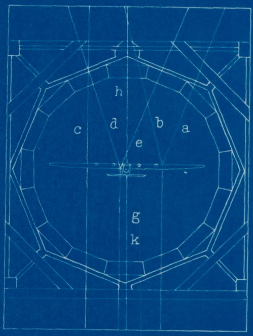
Fig. 7 Method of connecting model (rear view) with three-component balance, looking toward entrance cone.
