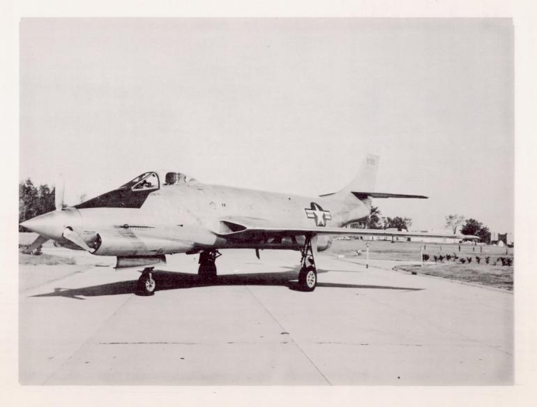
Figure 1.- The McDonnell XF-88B propeller research vehicle with test propeller.
