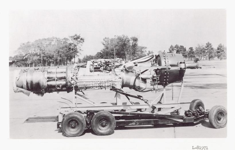
Figure 2.- The T-38 turboprop engine showing the power section and special gearbox.
