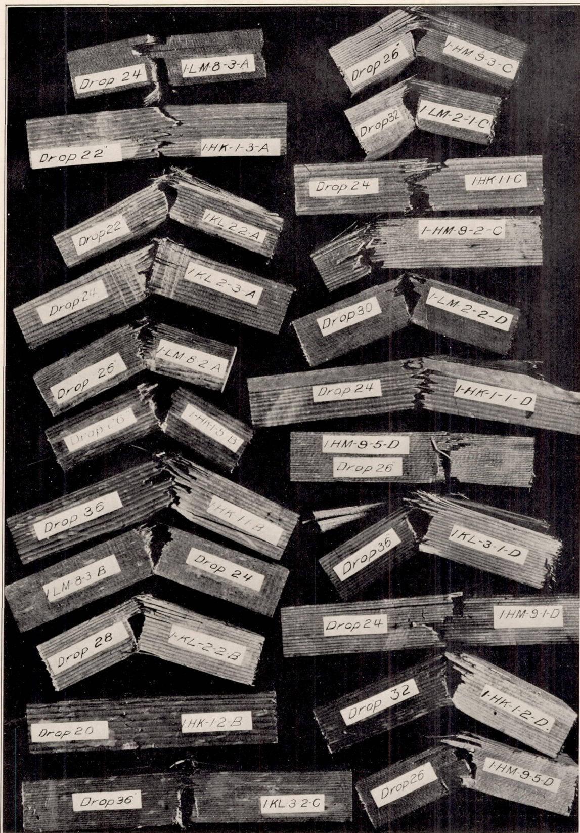
PLATE I.—FAILURES OF IMPACT-BENDING SPECIMENS, SITKA SPRUCE, KILN RUN 148.
