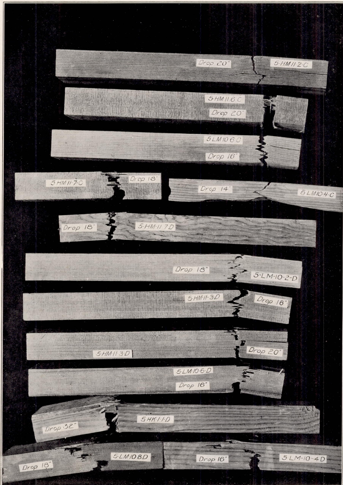
PLATE III.—FAILURES OF IMPACT-BENDING SPECIMENS, SITKA SPRUCE, KILN RUN 148.
