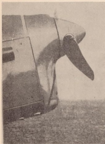
Figure 39.- Nose of Caudron 366 "Atalante" 217 hp. Regnier, fitted with Levasseur manually operated propeller. (Note forward tilt of blade).
