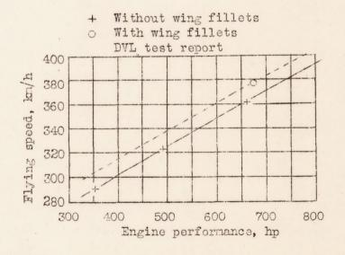
Figure 9.- Horizontal speed versus engine performance.
