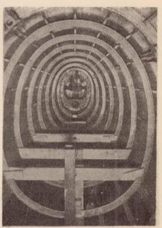
Figure 5.- Interior view of fuselage.
