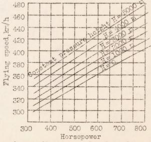
Reduced according to sea level performance of the He 70 in the DVL test flights. G= 3350 kg.
