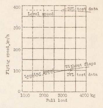
Figure 10.- Landing and horizontal speed versus full load.
