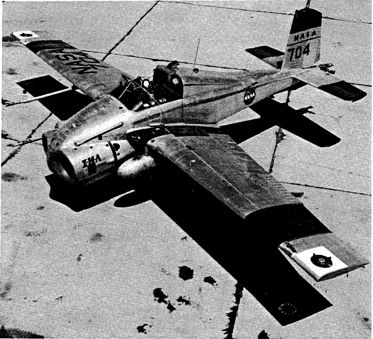
Figure 11. X14-A aircraft with tip-driven roll-control fans installed on wing tips.
