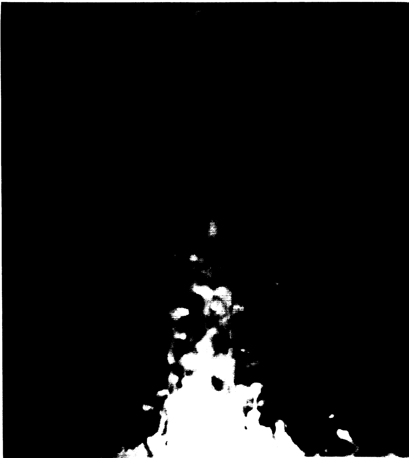
Figure 3. "Fingers" of polymer in a solution of methacrylic acid and benzoyl peroxide. The experiment was performed in a 2.2 cm (i.d.) tube but only the central 1-cm wide region is shown. Ambient temperature was 26 °C. [Benzoyl peroxide] = 1.0 g/100 ml.
