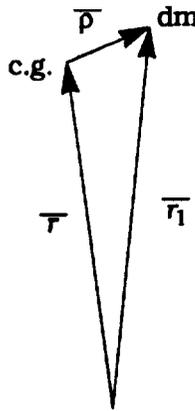
Figure 1 Position of a Particle of Mass in the Body Axis System
