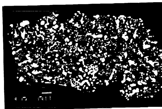
Figure 2. Ilmenite from mare soil 75061, reduced at 1050°C
