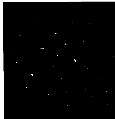
FIGURE 10.—Laue diffraction pattern of the enzyme protein crystal lysozyme in a quartz capillary.
