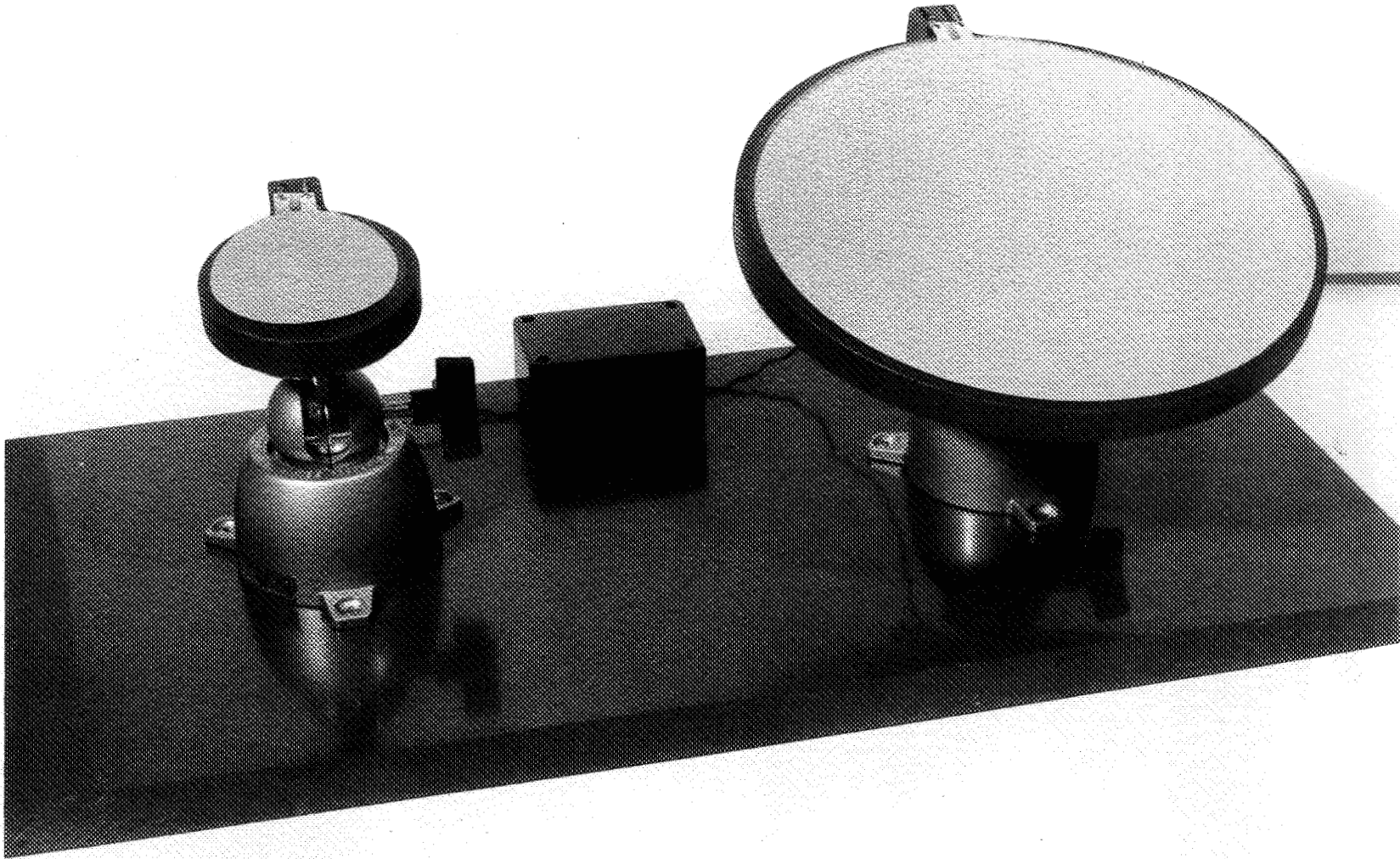
Figure 5. The NESDIS foil disdrometer sensors of 3-inch and 9,5-inch diameter mounted for testing. Mounting plates are adjustable to permit the correct pitch for water runoff.
