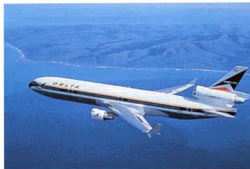
Winglets are in airline passenger service on the McDonnell Douglas MD-11 trijet, pictured here in Delta Air Lines livery.
