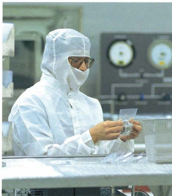
WSTF performs a wide range of services for its industry clients, among them servicing of parts used on oxygen systems — cleaning, repairing, testing and packaging, all conducted in a high technology clean room environment
