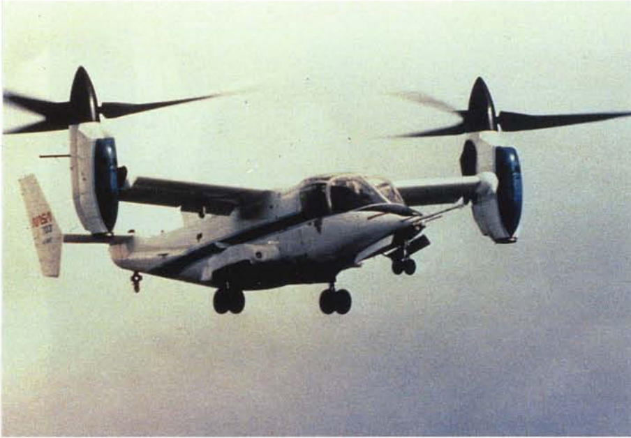
The NASA/Army XV-15 tiltrotor research craft is finding new utility as a flight test bed for advanced proprotor systems designed to minimize noise levels of tiltrotor aircraft.
