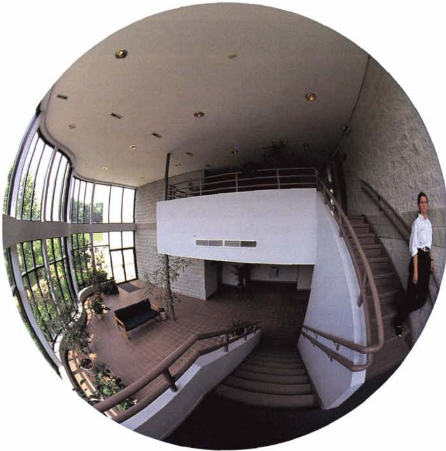
Surveillance of an apartment building lobby is one of many Omniview applications. A video image viewed through a wide angle fisheye lens would be badly distorted as shown at left, but Omniview removes the distortion and presents a corrected "flat" view on the monitor; note the distortion of the staircase in the fisheye view and the corrected closeup below.
