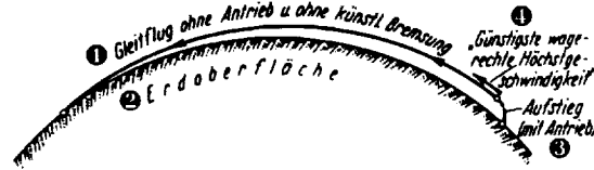
Figure 53. The most advantageous way of implementing an "express flight at a cosmic velocity" is as follows: the highest horizontal velocity is—corresponding to the distance—selected so large ("optimum horizontal velocity") that the entire long-distance trip can be made in gliding flight without power and without artificial braking (see Figure 50 for a diagram).
