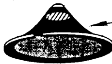
Maglev crew transfer pod is NASA Tension Aeroshell (e.g., see NASA TN-D-2994)
