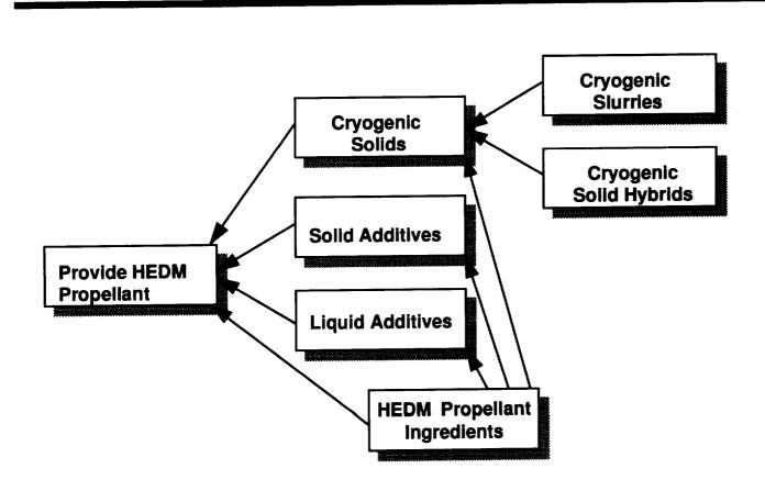
Propellants developed in the HEDM program range from near term application additived to LOX/RP-1 to very far term propellants, such as metallic hydrogen. One promising technology is in the area of cryogenic solid hybrid motors consisting of mixtures of energetic molecular systems, such as ozone, in "standard" propellants, such as oxygen. These mid-term technologies have the capability to provide 5 - 10 % improvements in specific impulse and density in the next 10 to 20 years.
