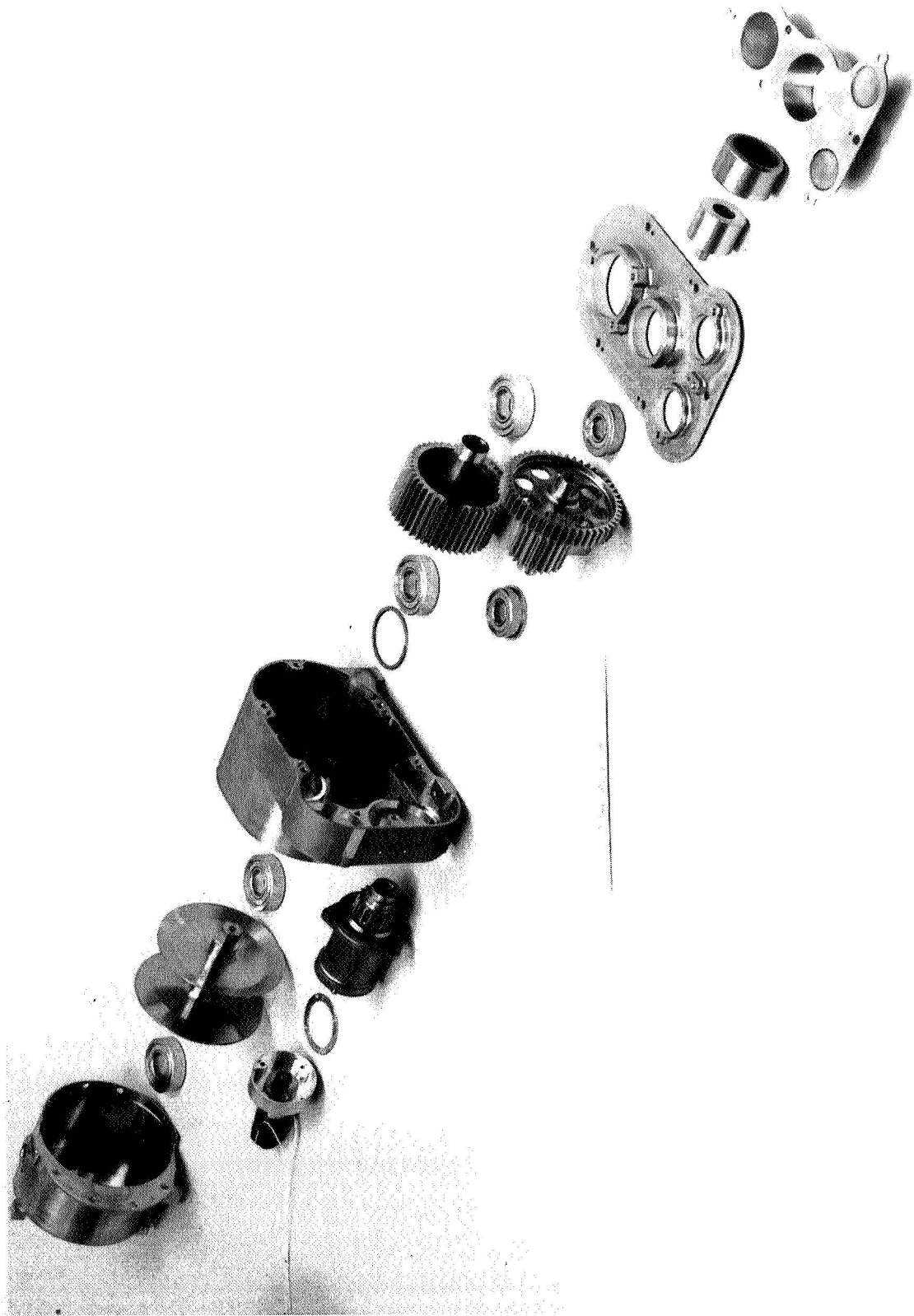
Figure 8 Airbag Retraction Actuator Exploded View
