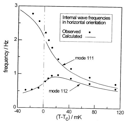
Figure 1. Internal-wave frequencies, measured (circles) and calculated (lines). The cell's axis was horizontal and the screen's torsion axis was vertical, so that the screen's motion was horizontal. The numerical calculations used the actual profiles derived from xenon's equation of state.
