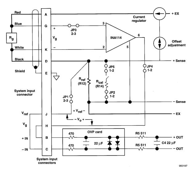
Figure 3. Four-wire gage connections.
