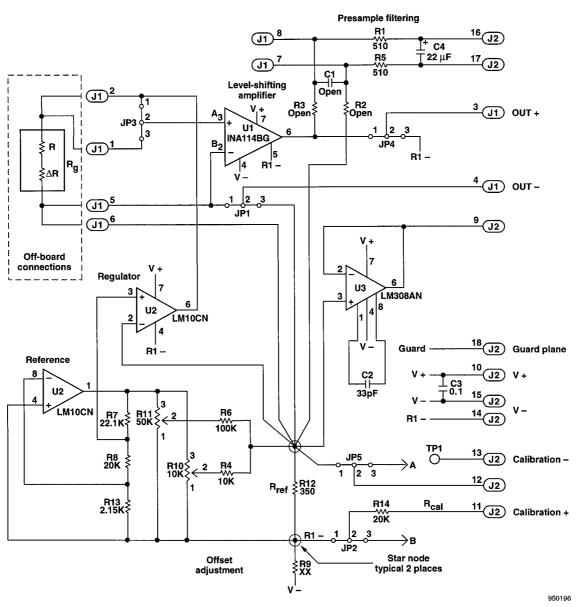
Figure 2. The production circuit schematic.
