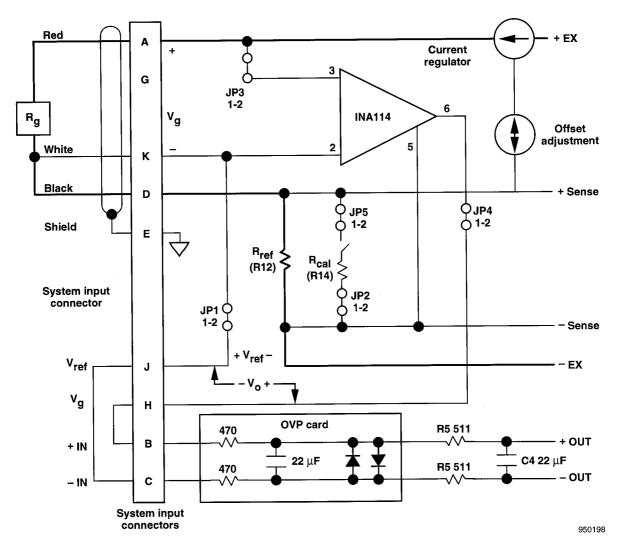
Figure 4. Three-wire gage connections.
