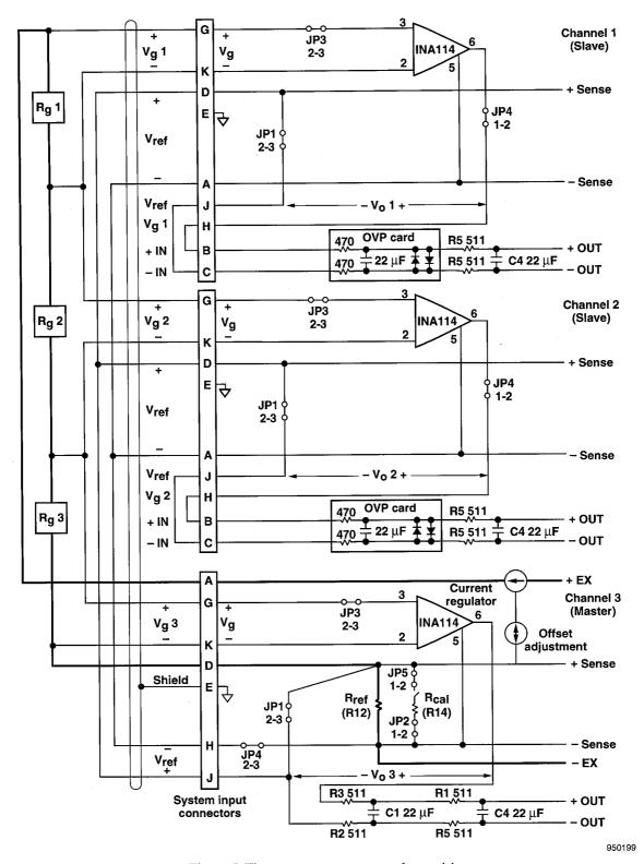
Figure 5. Three-gage rosette current-loop wiring.
