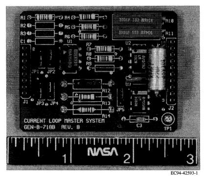
Figure 1. The DACS II current-loop printed circuit board.
