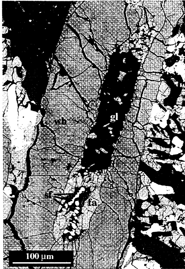
Figure 3. Backscattered electron photomicrograph of representative inclusion in phosphate. The host crystal is composed of whitlockite (wh), and the inclusion consists of fayalite (fa) and sulfide (sf) daughter crystals nucleating off the walls and ends of the inclusion within the interior glass (gl).
