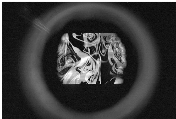
Figure 6.—Images through a viewing port into a chimney containing a soot-laden exhaust stream. The top panel shows a ruler giving the spatial scale in inches. The middle and lower panels are LII images produced with one and two single laser pulses, respectively, of soot within the post combustion exhaust.
