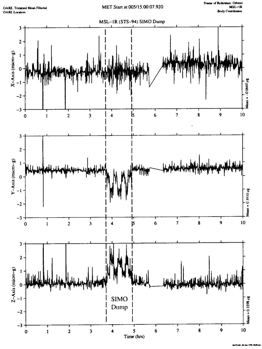
Figure 1. OARE Data Collected During a Simultaneous Supply and Waste Water Dump at MET 005/15:00.
