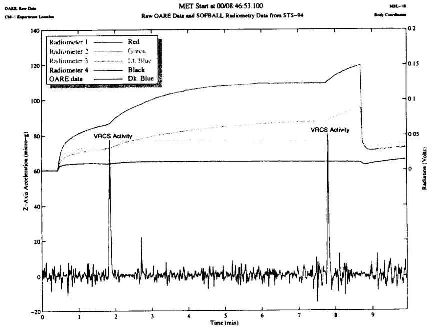
Figure 3. Raw (10 samples per second) OARE Data with SOFBALL Radiometry Data from STS-94, SOFBALL Test Point 14A. MET Start 007/08:46:53.
