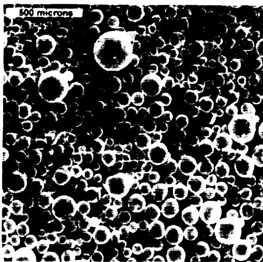
Fig. 3 Tin droplet dispersions as a consequence of applying ultrasonic ( f = 20 kHz) energy with a probe amplitude of (a) 64\mu\text{m} and (b) 137\mu\text{m} for \sim 1 minute.
