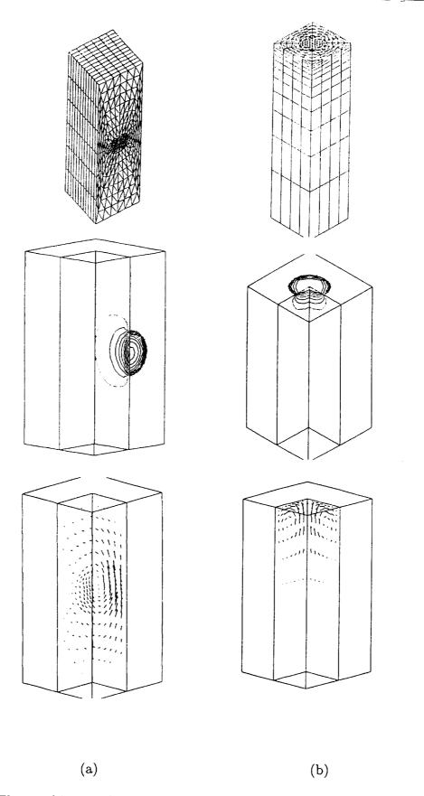
Figure 1. The meshing used, the isotherms and the fluid velocity vectors for (a) side heating, and (b) top heating.
