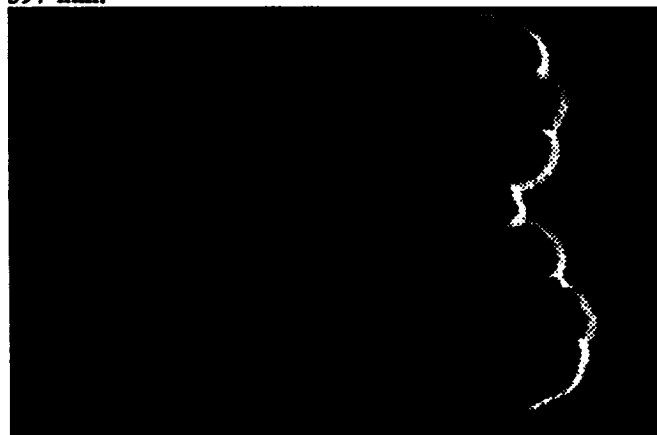
Figure 4. Images of flames in Hele-Shaw cells: (d) 7.1% C 2 H 2 in air, horizontal propagation, 0.30 s after ignition. Flame propagates from left to right. Field of view is 394 mm x 597 mm.
