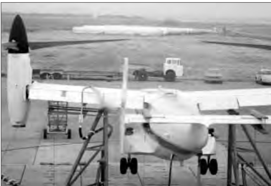
Top: Figure 56. Flow visualization near the XV-15 wing tips. (Ames Photograph AC85-0804-49)
