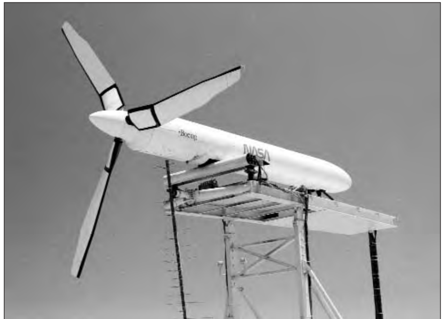
Figure 63. Advanced Technology Blades proprotor mounted on the test apparatus at the Ames Research Center Outdoor Aerodynamic Research Facility. (Ames Photograph AC84-0498-2)
