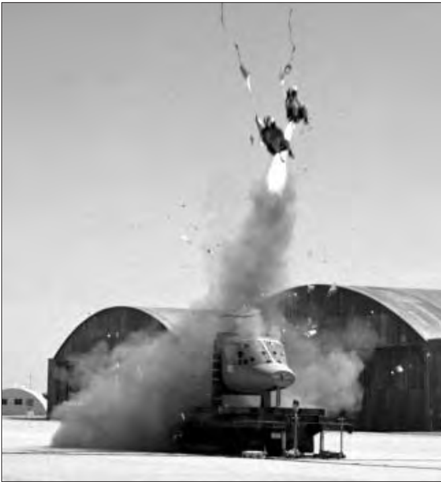
Figure 41. Simultaneous static test firing of XV-15 ejection seats. (Ames Photograph AC75-1602)
