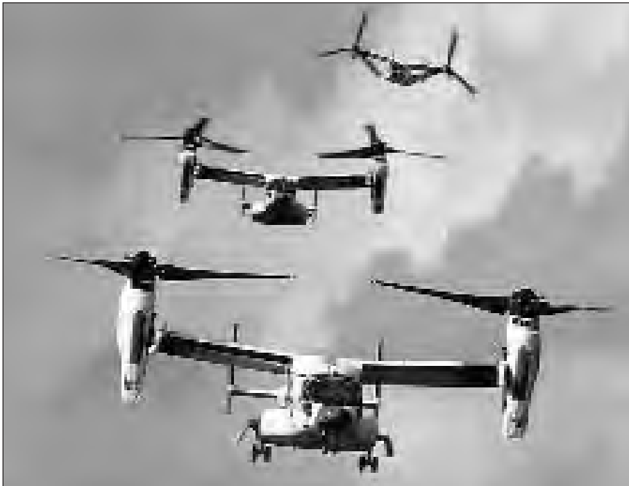
Figure E-14. Composite photograph showing V-22 Osprey in hover, conversion, and airplane mode flight. (Bell Photograph 039956)
