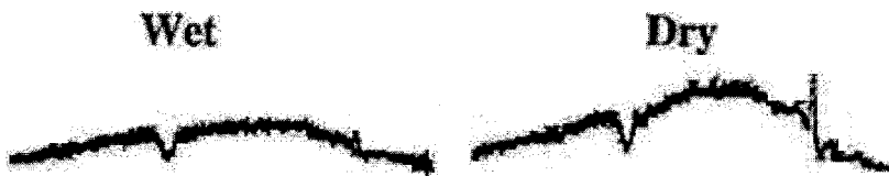
Figure 5. Raman spectra of dry and wet soil samples obtained under 514.5 nm laser excitation, in the wavelength region 800-450 nm.
