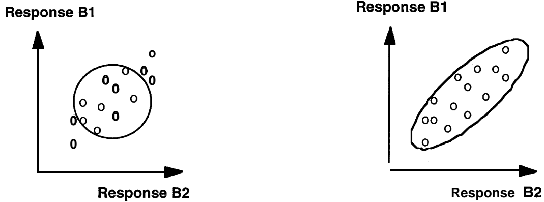
Figure 3. Two dimensional representation of a spectral response at binds 1 and 2. Part a does not take into consideration second order statistics, it assumes no correlation among the bands. Part b does take into consideration second order statistics, with no assumption about the correlation among the bands.
