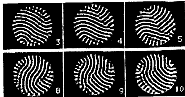
Figure 1: Snapshots of experimentally observed Küppers-Lortz state in buoyancy-driven convection (top view) [3].
