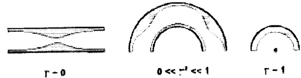
Figure 7 Types of liquid accumulation in the bend of the vapor line for various values of \Gamma with \delta < 0.1 .
