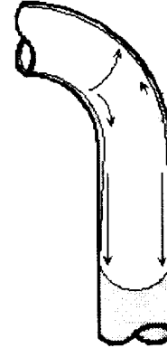
Figure 6 Vectors representing magnitude and direction of liquid film flow in CHT experiment.
