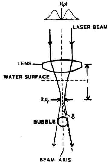
Figure 4: Optical trapping of a bubble in a focused beam with the divergence greatly exaggerated. The irradiance profile  $I(\rho)$  at top is that for a pure  $TEM_{01}^*$  mode while, for the actual mode, the minimum in center was less pronounced.
