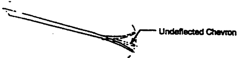
Flipper Chevrons Located on External Plug Nozzle (Alternating Chevrons Penetrating the Core/Fan Flows)
