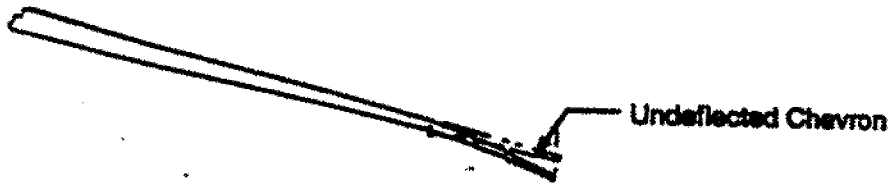
Flipper Chevron Located on External Plug Nozzle (All Chevrons Penetrating the Core Flow)
