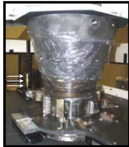
Figure 10: A close-up of the specialized tooling plate being used to bond the belly band. The arrows point to the plumb bob used to ensure angular position. (right)
