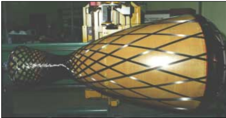
Figure 6: Wet winding of carbon/epoxy over silica/phenolic liner covered with film adhesive.
