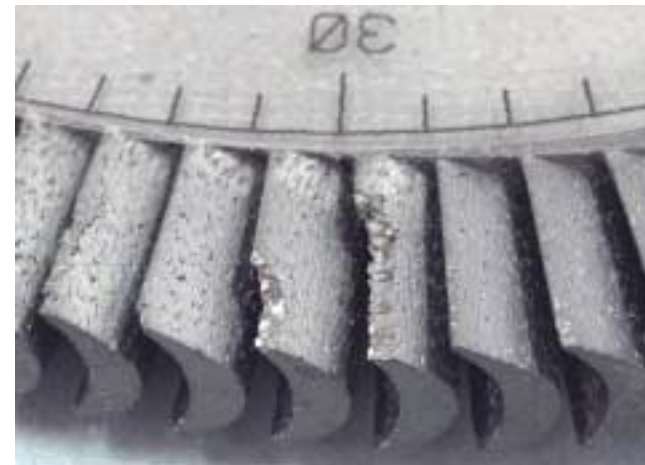
Typical trailing edge damage on the quasi-isotropic blisk
