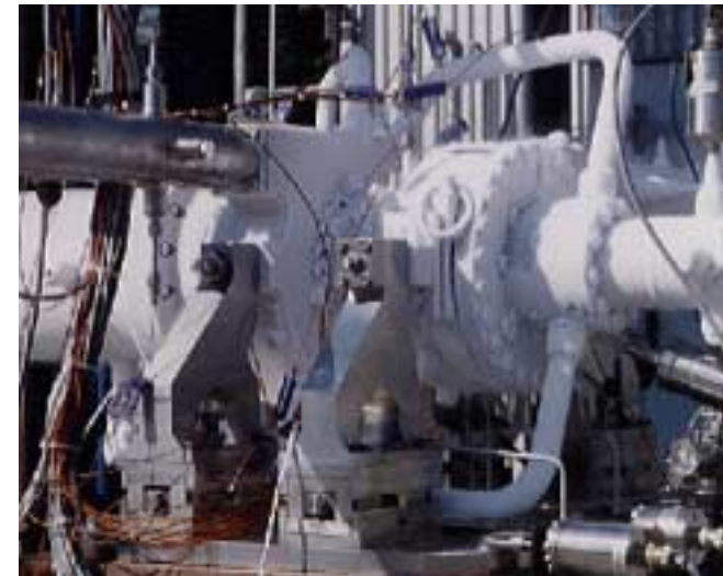
Simplex Turbopump Test Bed at NASA MSFC during chill down prior to testing.
