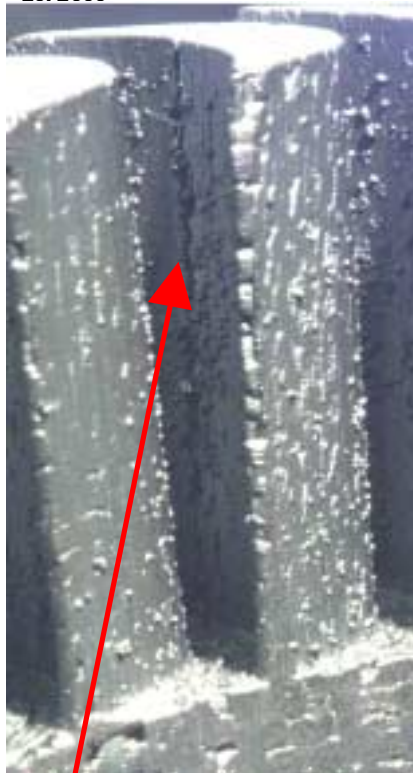
Cracked Polar Blade
