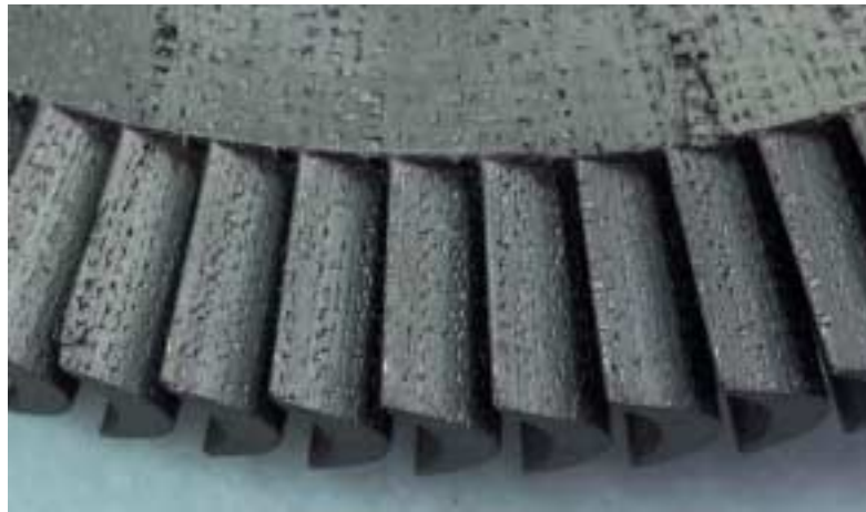
Nominal appearance of C/SiC blisk surface (Honeywell Advanced Composites, Inc.)
