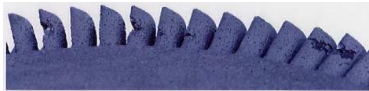
FOD impact pattern on Quasi-isotropic CMC blisk
