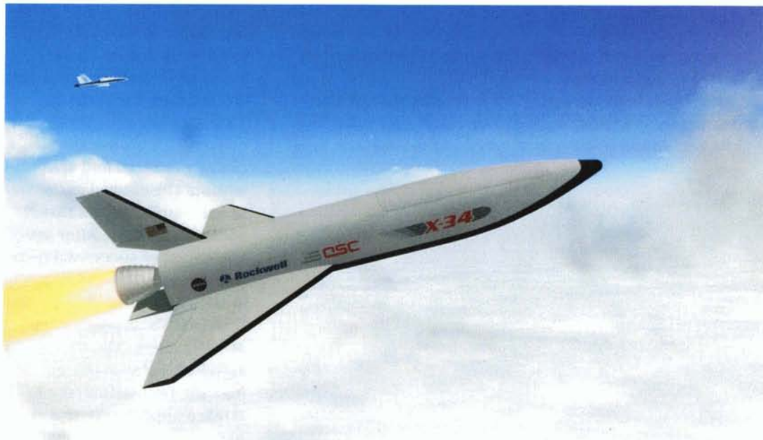
Being developed by Orbital Sciences Corporation and Rockwell International, the X-34 small reusable booster will be air-launched from a 747 transport; it will deliver a payload to orbit, then reenter the atmosphere and land on a runway.
