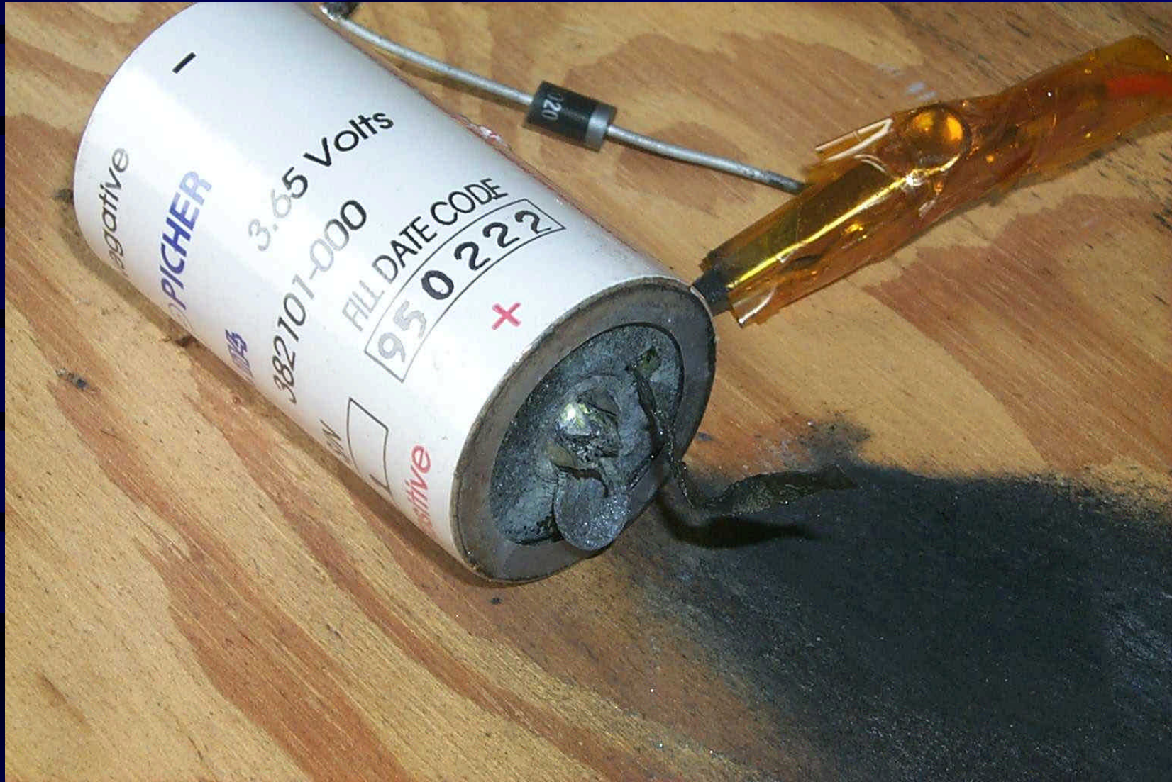
LTC-114 Cell Vented during 3A Over-Discharge
