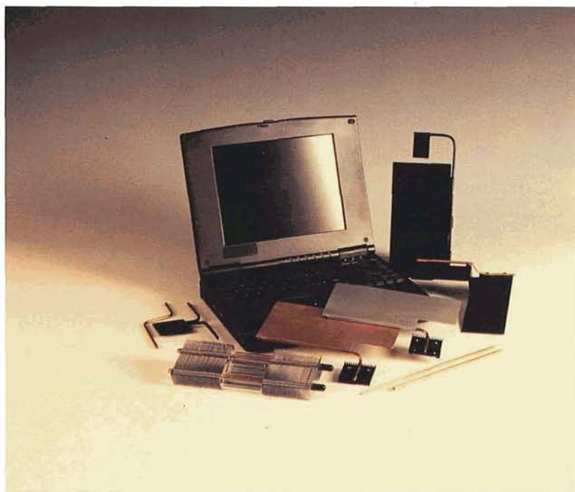
*NASA heat pipe technology used in spacecraft to keep hardware and critical electronics cool has found its way into notebook computers. Tiny heat pipes are in wide use to cool the main central processor chip.*
