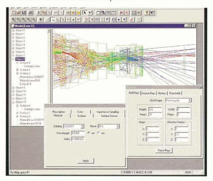
Lambda Research's TracePro software depicts rays of light moving through an optical system. In this instance, the blue light rays indicate the paths of unwanted stray light that can ruin an image. JPL-funded work helped put a new light on this unique software for a range of commercial applications.
