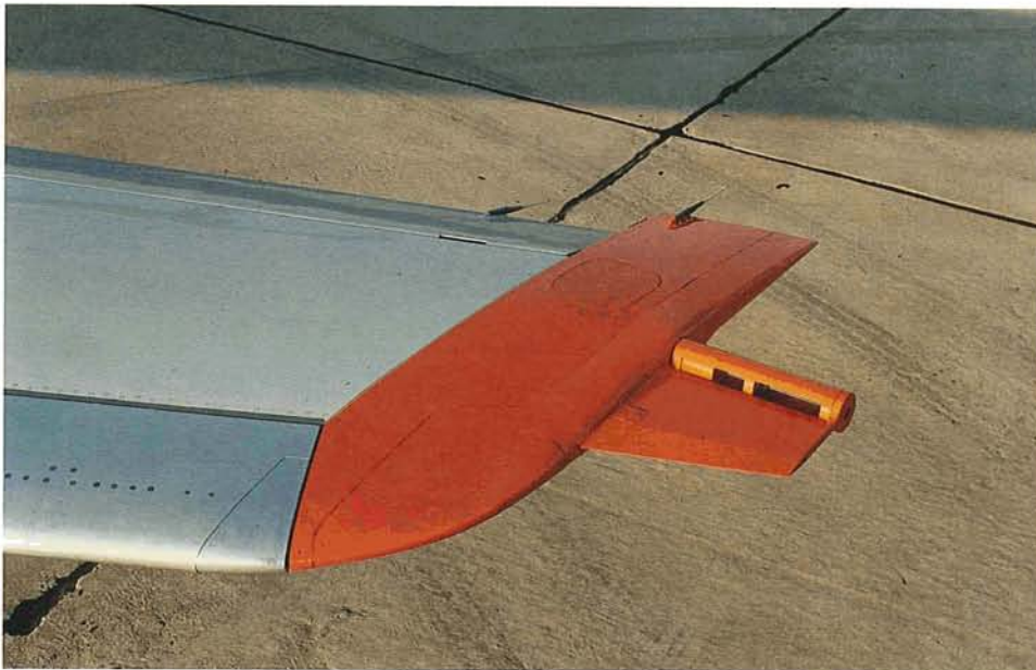
Dynamic Engineering Inc.’s Flutter Exciter mounts at the wing tips and tail tips of an aircraft to damp out structural vibrations.
