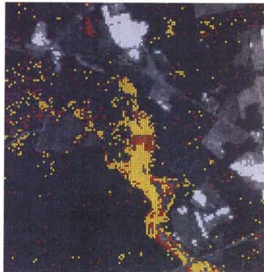
between normal satellite imagery (at left) and a subpixel processed image; the yellow/red area in the right image represents the additional information obtained by subpixel processing.
