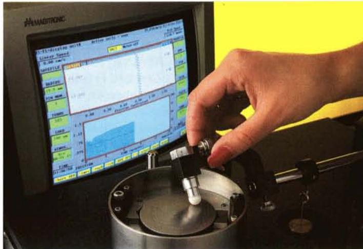
a wear groove on the surface of the disk. The system can be used to measure the coefficient of friction, the wear behavior between materials, and the integrity of thin films or coatings.
