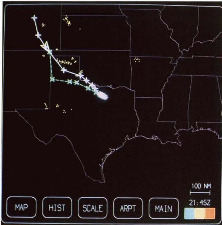
cost datalink. It is a two-way system that uplinks weather information to the aircraft and downlinks automatic pilot reports of weather conditions aloft.
