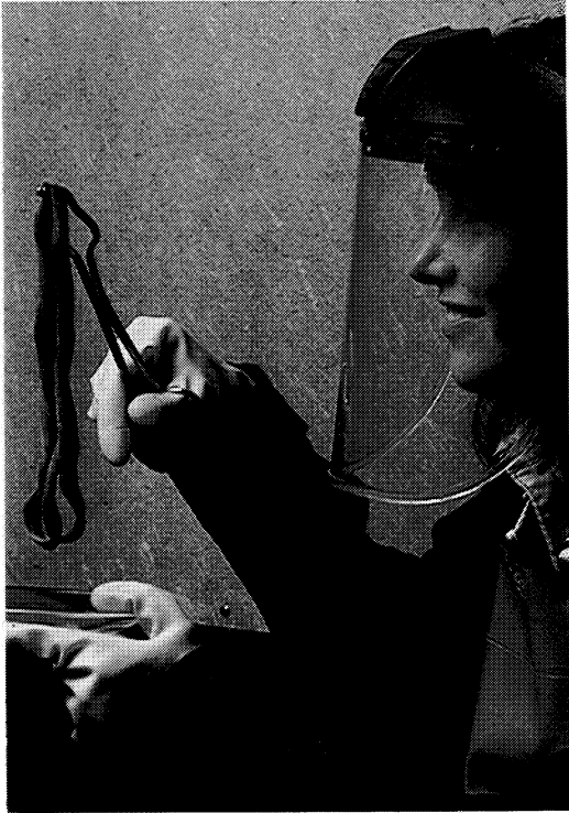
At left, a Celanese Corporation laboratory technician is acid bath-testing a batch of PBI fibers. Originally developed as material for fire resistant flight suits, the fibers are now being used in a widening range of civil applications.
