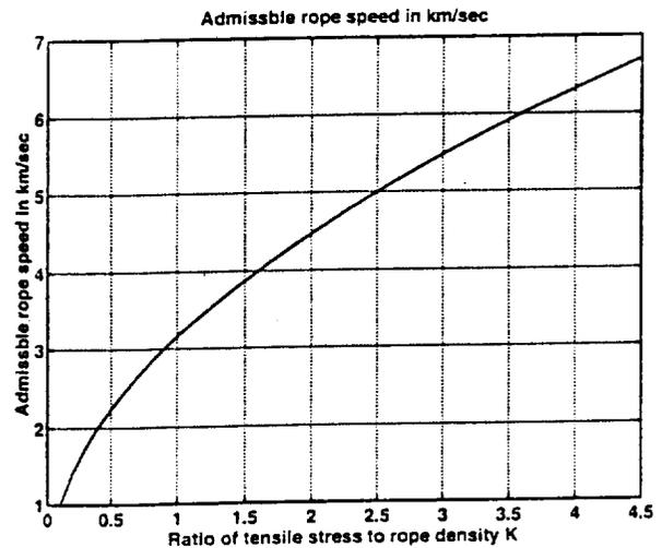
Fig.10. Admissible cable speed (in km/sec) via the ratio of a tensile stress to cable density (coefficient  $K$ ).
