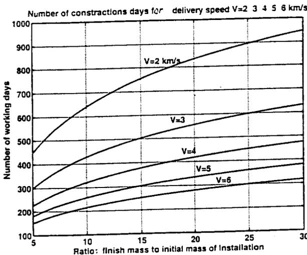
Fig.12. Number of working days via a ratio of a finish mass to an initial mass of the installation for delivery speed  $V=2-6$  km/sec.
