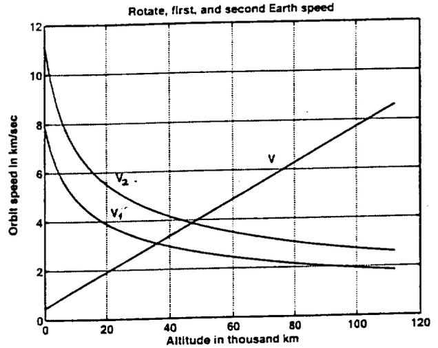
Fig.9. Rotate, first, second Earth speed (in km/sec) via altitude (in thousand km).
