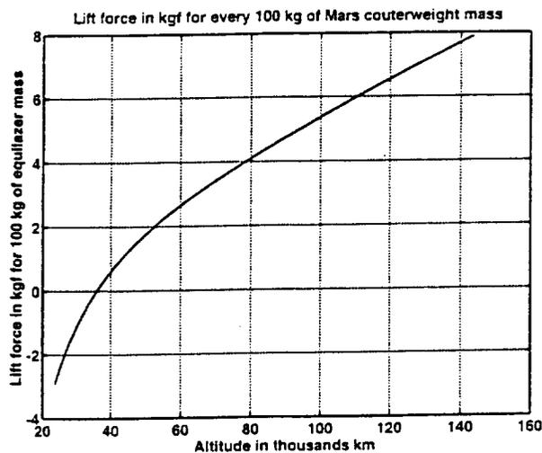
Fig.16. Lift force (in kgf) via altitude (in thousand km) for every 100 kg of Mars equalizer mass.
