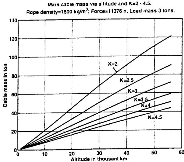
Fig.15. Mars cable mass via altitude (in thousands km), a cable density  $1800 \text{ kg/m}^3$  and a load mass of 3 tons.
