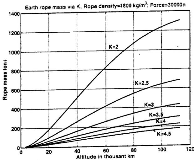
Fig.4. Cable mass in tons via counterweight altitude for Earth surface force of 3 tons, cable density 1800 kg/m<sup>3</sup>, and K=2-4.5 .
