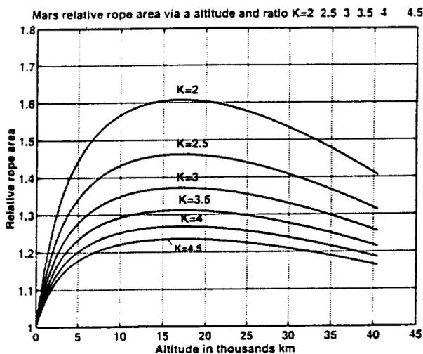
**Fig.14.** Mars relative cable area via altitude and coefficient  $K=2-4.5$ .
