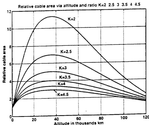
Fig.3. Relative cable area via altitude (in thousands km) for coefficient  $K=2-4.5$  .
