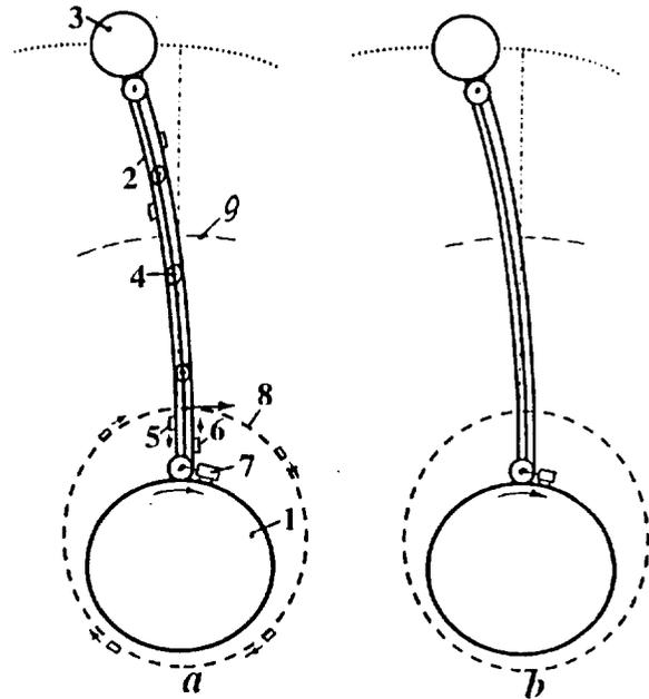
**Fig.1a,b.** The suggested Space Transport System. Notations: 1 – Rotary planet (for example, the Earth); 2 - suggested Space Transport System ; 3 - equalizer (counterweight); 4 - roller of Transport System; 5 - launch space ship; 6 - a return ship after flight ; 7 – engine of Transport System; 8 – elliptic orbit of tourist vehicles; 9 - Geosynchronous orbit. *a* – System for low coefficient *k*, *b* – System for high coefficient *k*.
