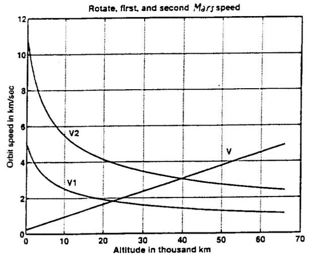
Fig.18. Rotate, first, and second Mars speed via altitude (in thousand km).
