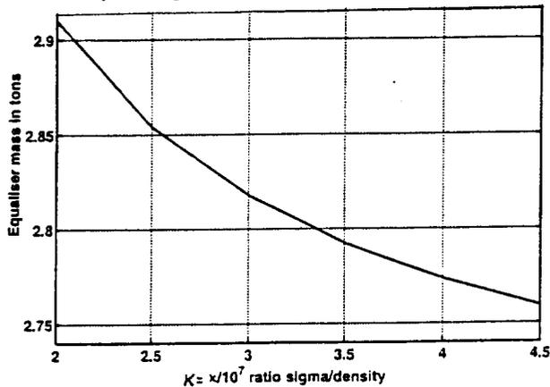
Fig.17. Mars counterweight mass (in tons) via the coefficient  $K = 2-4.5$  for altitude 50,000 km and the force 100 kgf.
