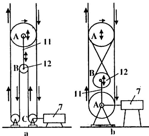
Fig.2a,b. Two mechanisms for changing the rope length in the Transport System (They are same for the space station). Notations: 11 - the rope which is connected axis A,B. This rope can change its length (the distance AB); 12 - additional rollers.
