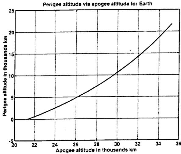
Fig.7. Perigee altitude (in thousands km) via disconnected (apogee) altitude of a space ship.
