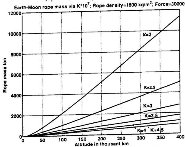
Fig.21. The Earth-Moon cable mass via altitude (in thousands km) for cable density  $1800 \text{ kg/m}^3$ , delivery mass 3 tons, and the coefficient  $K=2-4.5$ .
