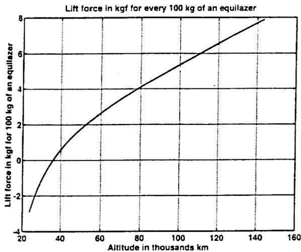
Fig.5. Lift force (in kgf) via altitude (in thousands km) for every 100 kg of a counterweight (equalizer).
