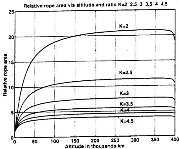
Fig.20. Relative cable area via a maximum altitude to the Moon (up 400,000km) and the coefficient  $K=2 - 4.5$
