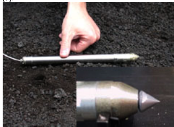
Figure 1. PLUTO mole demonstrated on Mt. Etna in Sept. 2002. The inset lower right shows the sampling device.
