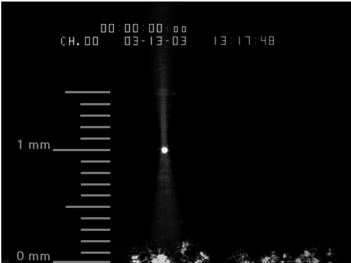
Figure 3.—Composite photograph showing a single 100 \mu\text{m} glass sphere with the relative height above the glass plate and position within the focused beam shown.
