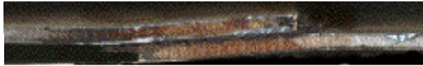
Figure 6. A tested aluminum lap shear specimen showing deformed joint after metal failure.
