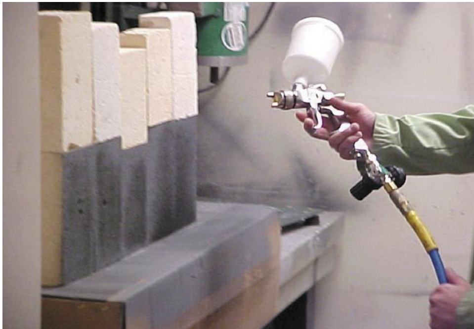
Samples are sprayed with Emisshield ST-1 in Wessex Incorporated's laboratory.
