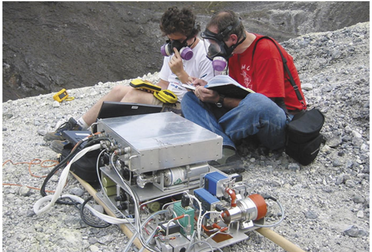
Researchers record data as the hazardous gas detection system is used to analyze the toxic gases produced by active vents, called fumaroles, in the Turrialba volcano in Costa Rica.
