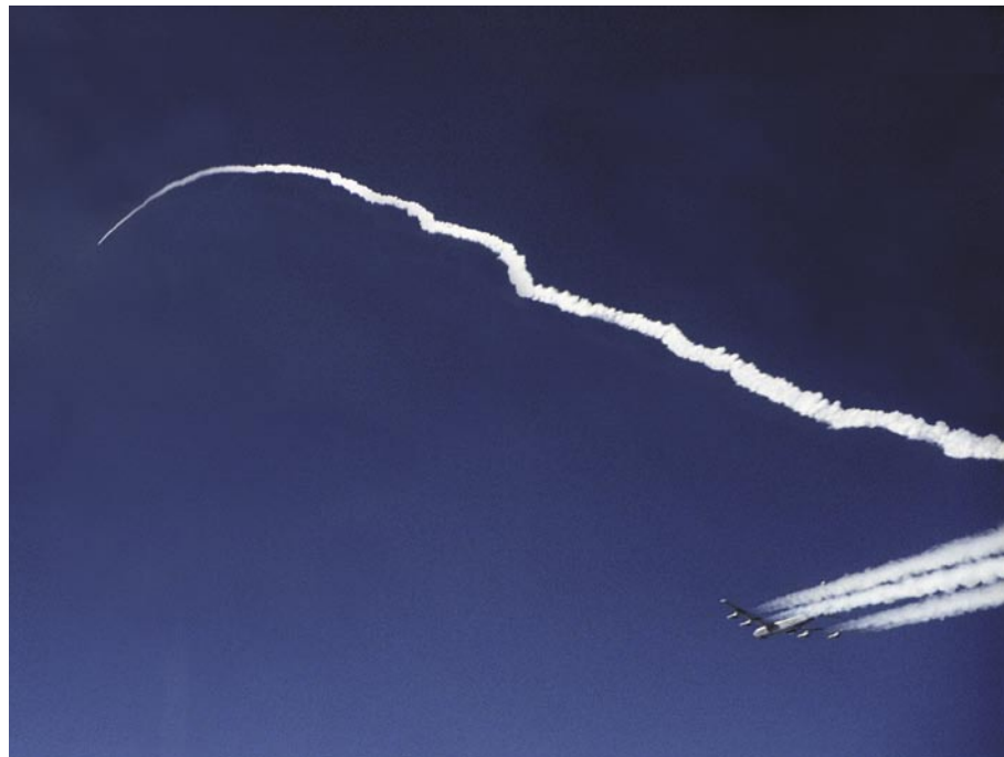
The X-43A hypersonic research aircraft and its modified Pegasus booster rocket accelerate after launch from NASA's B-52B launch aircraft over the Pacific Ocean.
