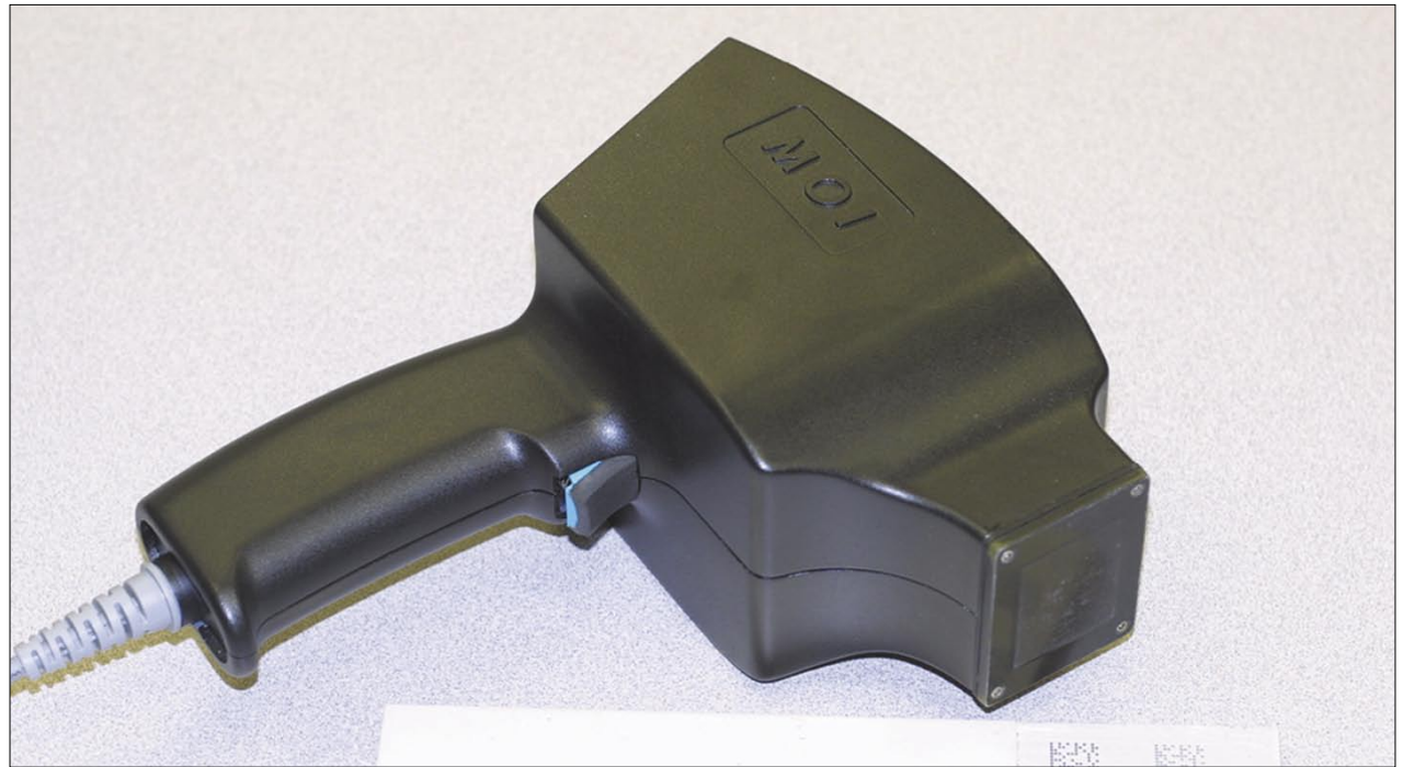
The Magneto-Optic Imager reads and decodes magnetic matrix symbols that are obscured by paint or other coatings.
