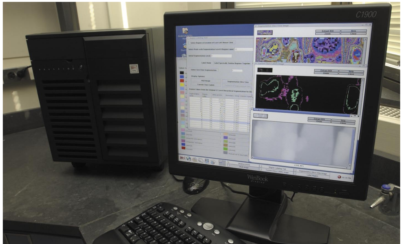
As an open workstation, Med-Seg™ is composed of a front-end terminal for segmentation feature extraction, pattern recognition, and classification of medical images, including computed tomography scans, positron emission tomography scans, magnetic resonance imaging, and ultrasound.
