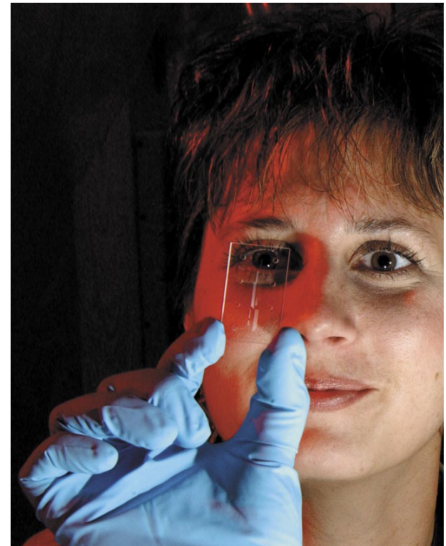
Dr. Lisa Monaco, the project scientist for the Lab-on-a-Chip Applications Development program, examines a lab on a chip. The small dots are actually ports where fluids and chemicals can be mixed or samples can be collected for testing.
